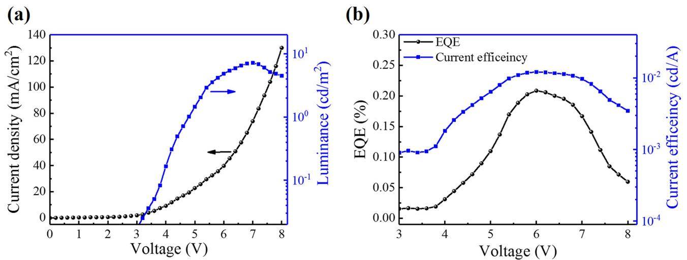
**Figure 3.** (a) Current density and luminance versus voltage, and (b) external quantum efficiency and current efficiency versus voltage for the CsPbI<sub>3</sub> QD LEDs.
