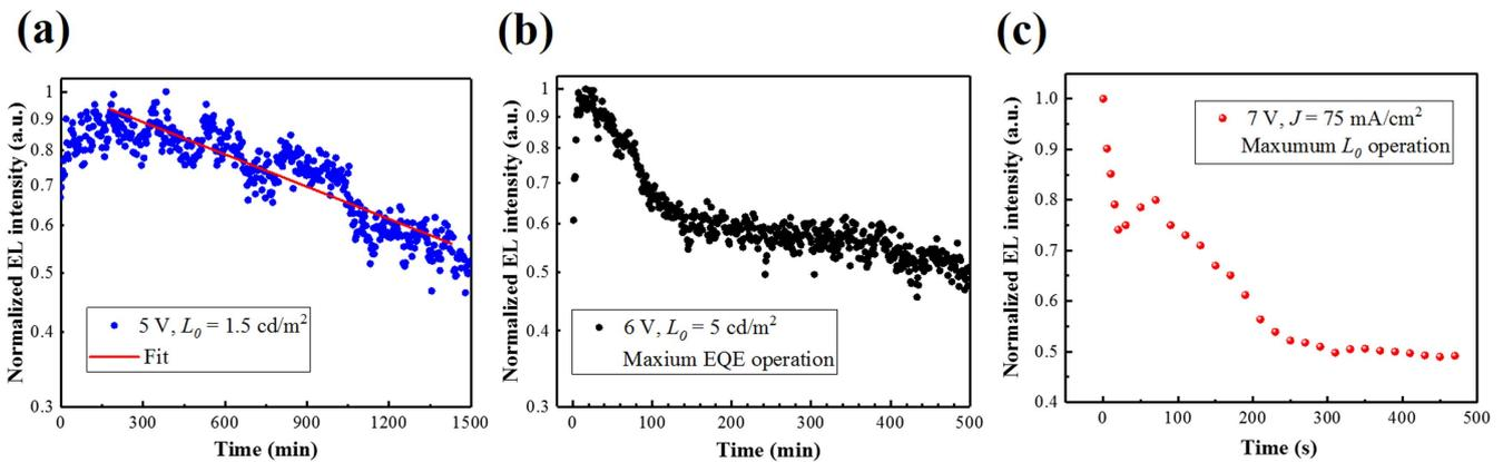
**Figure 5.** Stability characterizations of the device under (a) low bias of 5 V, (b) 6 V bias where maximum EQE is achieved, and (c) high bias and current injection condition (7 V,  $J = 75 \text{ mA cm}^{-2}$ ), where maximum luminance is reached. (a) and (b) are in logarithmic scale and (c) is in linear scale. The measurements were performed at room temperature under ambient conditions.
