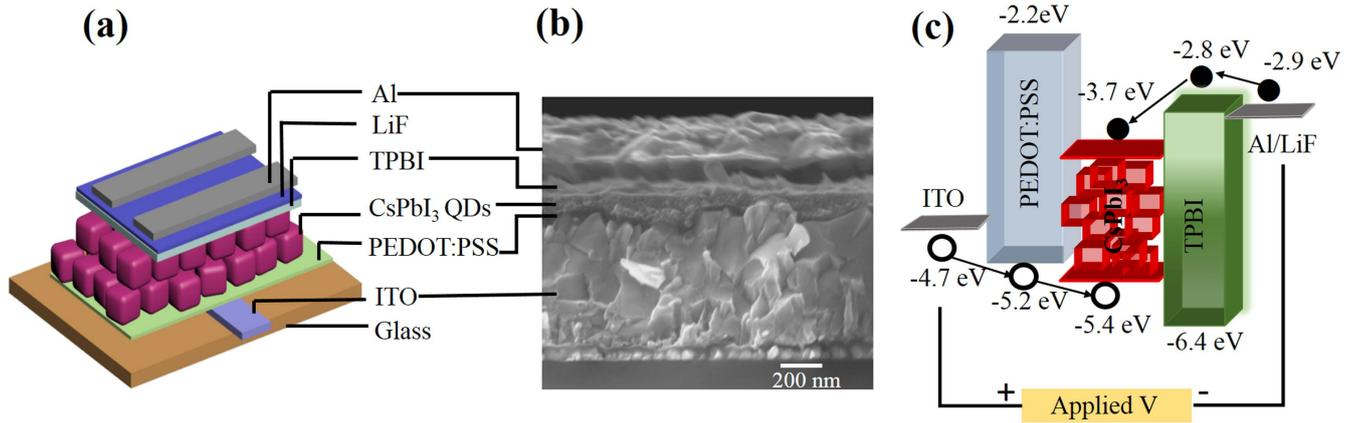
**Figure 2.** (a) Schematic diagram of the CsPbI<sub>3</sub> QD LED device structure. (b) The cross-section view SEM image of the fabricated device. (c) Energy band diagram of the LED device.
