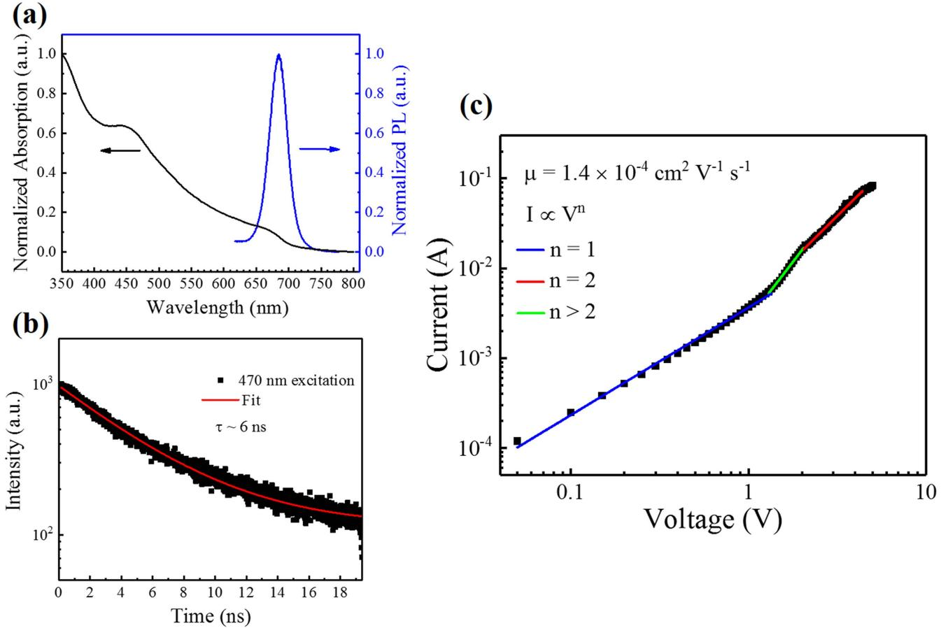
**Figure 1.** Characterizations of the CsPbI<sub>3</sub> QD film. (a) UV–Visible absorption and PL spectra. (b) Transient PL measurement. A lifetime of 6 ns was obtained from fitting the data. (c)  $I$ – $V$  measurement of a hole-only device in the dark condition for extracting the mobility in the CsPbI<sub>3</sub> QD film using a space charge-limited current method.
