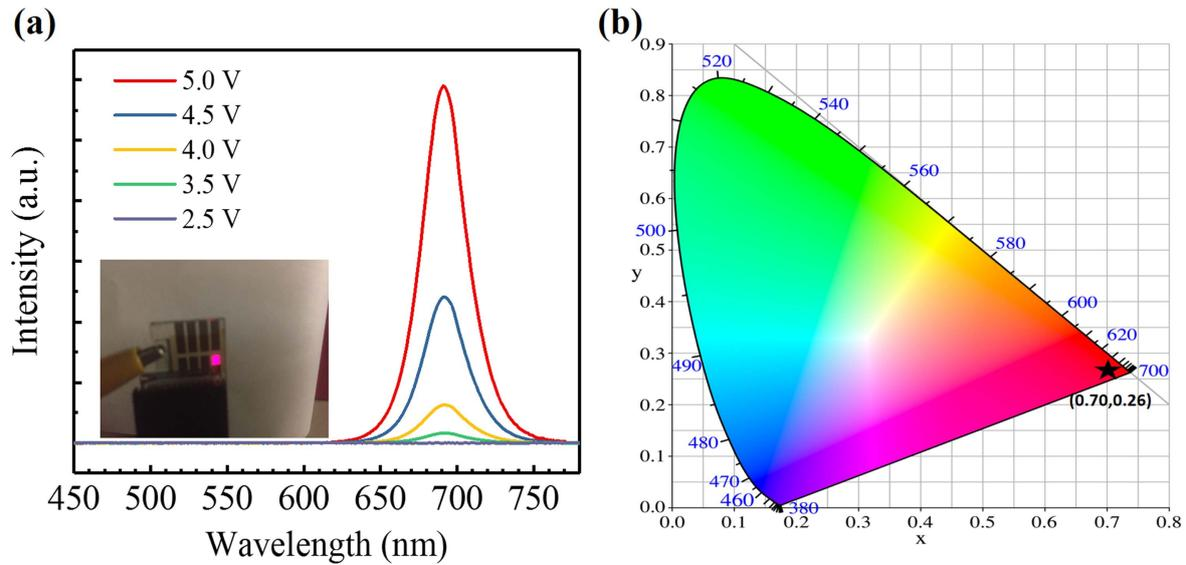
**Figure 4.** (a) EL spectra under different applied voltages. Inset: Photograph of the device in operation, showing red emission. (b) CIE coordinates of the emitted light from the CsPbI<sub>3</sub> QD LED.
